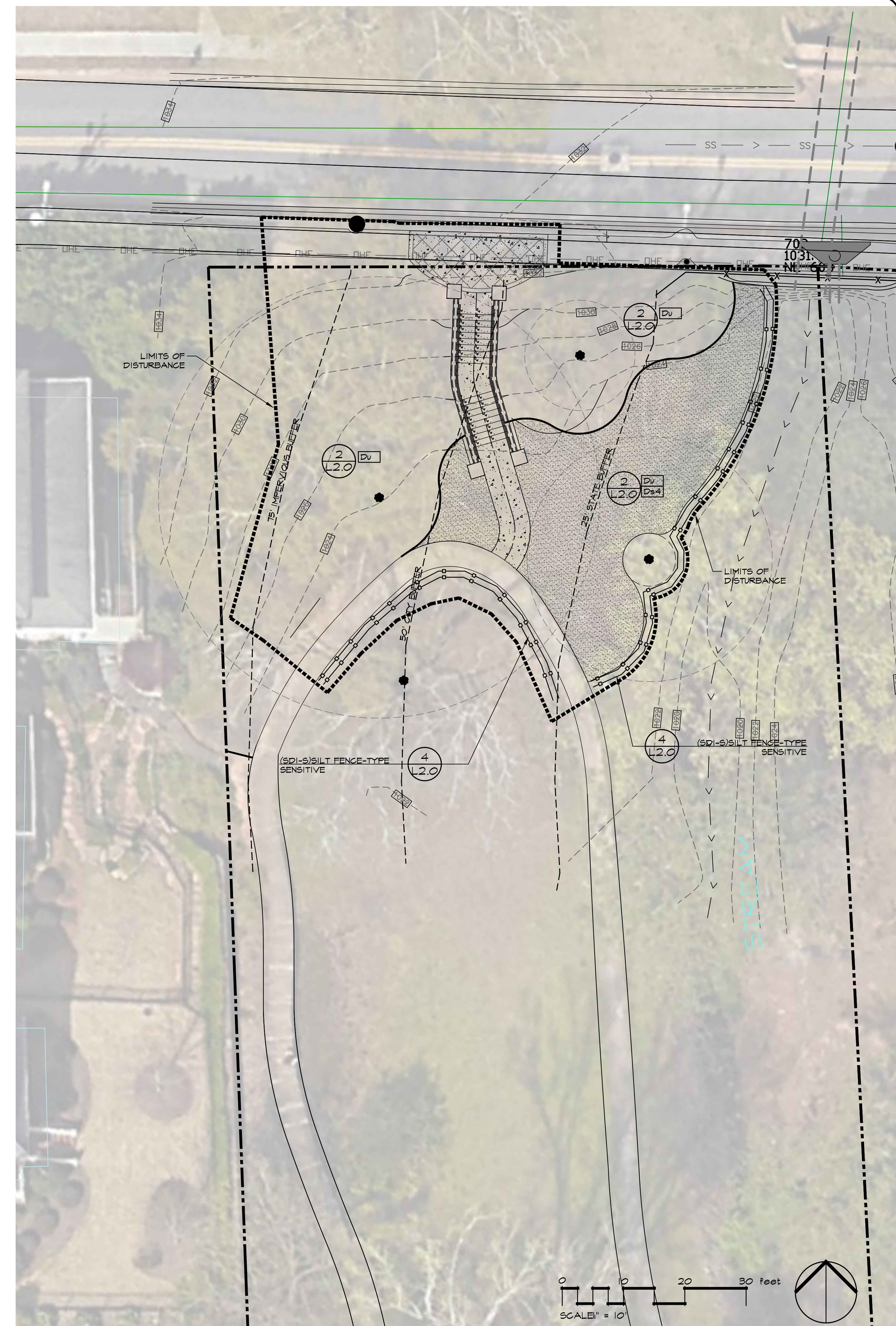
1 EROSION, SEDIMENT, AND POLLUTION CONTROL PLAN
