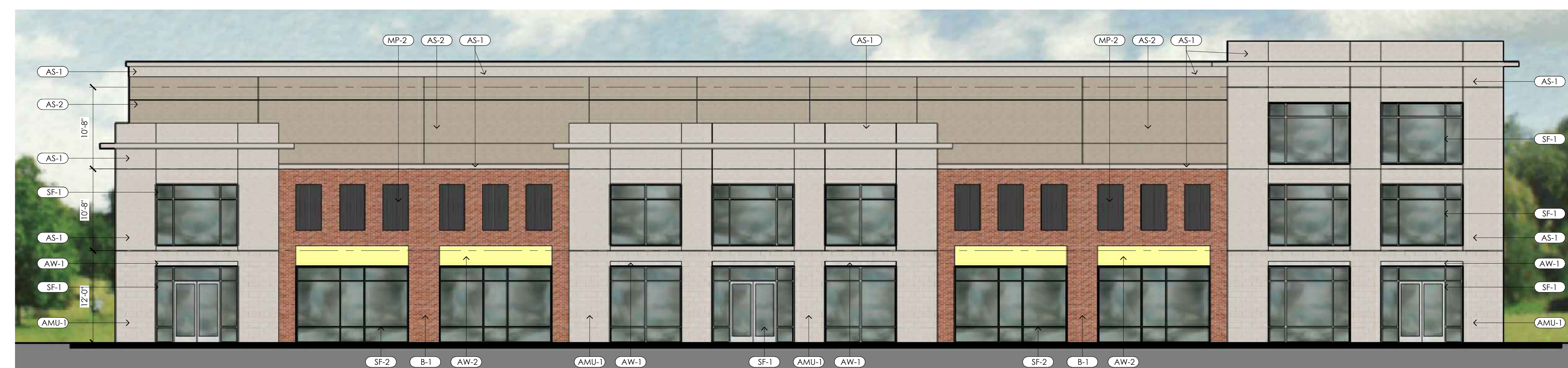
02 NORTH (SPRING ROAD) ELEVATION A2.1 1/8"=1'-0"
