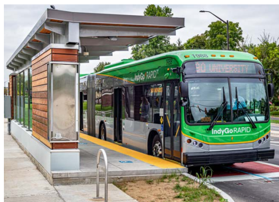
Example of a BRT vehicle that operates in a curbside running way stopped at a station featuring level boarding, a shelter, and bicycle parking.
