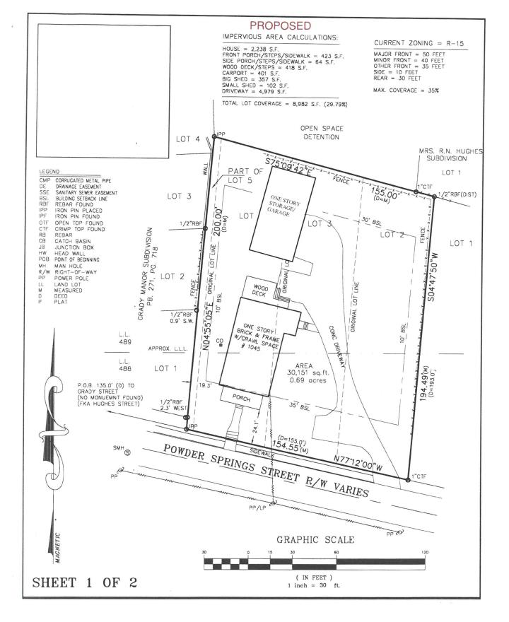
Proposed location to the Rear of primary structure holding the NW lines of both structures in plane, approximately 25' apart while maintaining rear and side setbacks.
