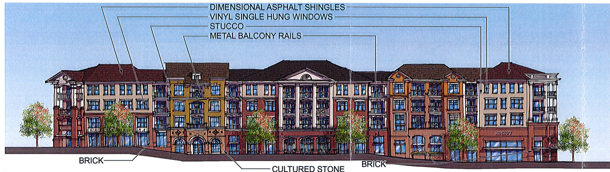
POD "B" - WEST ELEVATION
