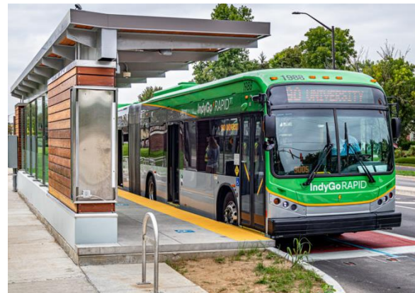
Example of a BRT vehicle that operates in a curbside running way stopped at a station featuring level boarding, a shelter, and bicycle parking.
